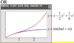
For  $1 \le x \le 2$ , the **graph** of  $y = x - \frac{1}{2}x^2 + \frac{1}{6}x^3$  deviates from that of  $y = \sin(\ln(1+x))$ .
